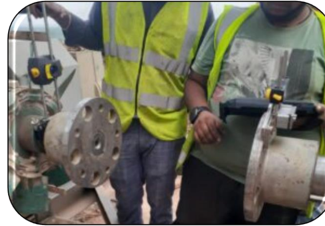
Laser alignment at site
